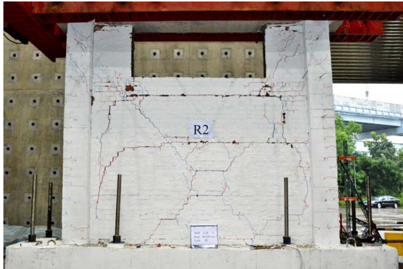
側位移比1.25%，牆體受擠壓損壞呈現蜘蛛網狀裂隙
